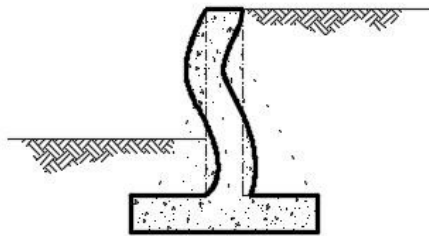
OVERSTRESS OF WALL
